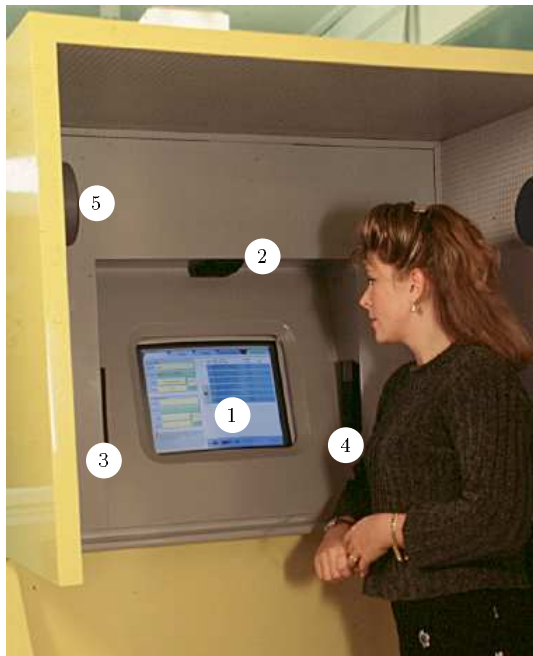
Fig. 1 The LIMSI MASK data collection kiosk, (1) touch screen, (2), (3) and (4) are microphones, and (5) loudspeaker.
